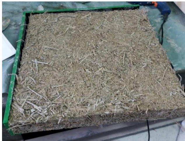
Fig.2. Insulation panel of Miscanthus fibers with cementitious binder [14,15]
